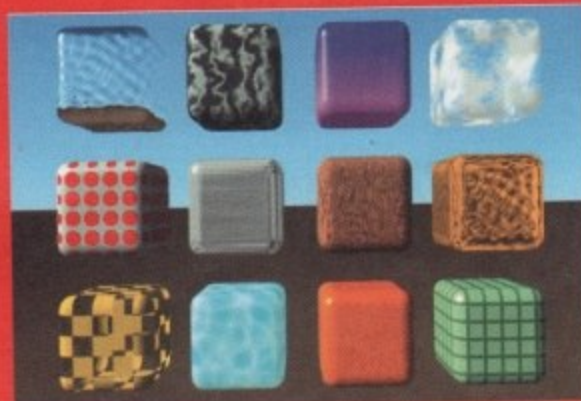
The Lightwave textures example scene is a good test of speed. Standard A4000 speed is 17 minutes 50 seconds, whereas Cyberstorm bangs out a frame in only 4 minutes 10 seconds.
